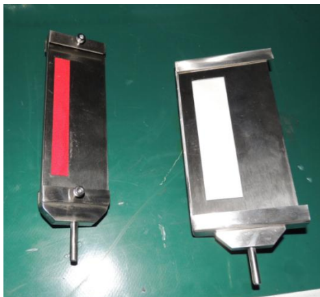
Lock sample holder's screws to fix it
