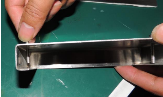
Loose sample holder's screws a little.
